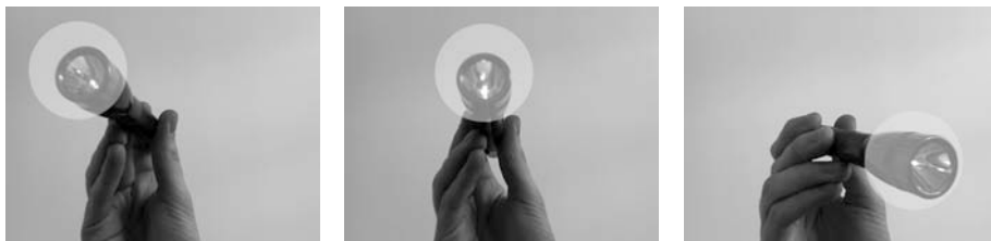
Example 4. Tracks the brightest object in each video frame by calculating the brightest pixel. The light from the flashlight is the brightest element in the frame, therefore the circle follows it.
