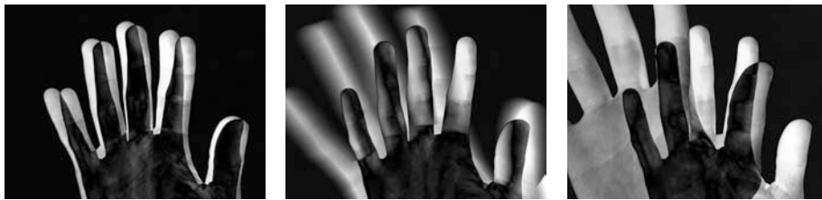
Example 2. Detects the presence of someone or something in front of the camera by comparing each video frame with a previously saved frame. The change is visualized and is calculated as a number.
